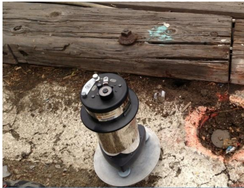
Figure 2.1 Worden Gravimeter and one of our Benchmark stations (located within the reddish circle)
