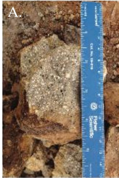
Figure 5: A) Young Group Volcanics are dominated by dacitic lavas and tuffs, located along the rim of the caldera and on the flanks of the volcano. Primary mineralogy consists of quartz, plagioclase and biotite. Densities of rocks within this unit are lower than the old group.
