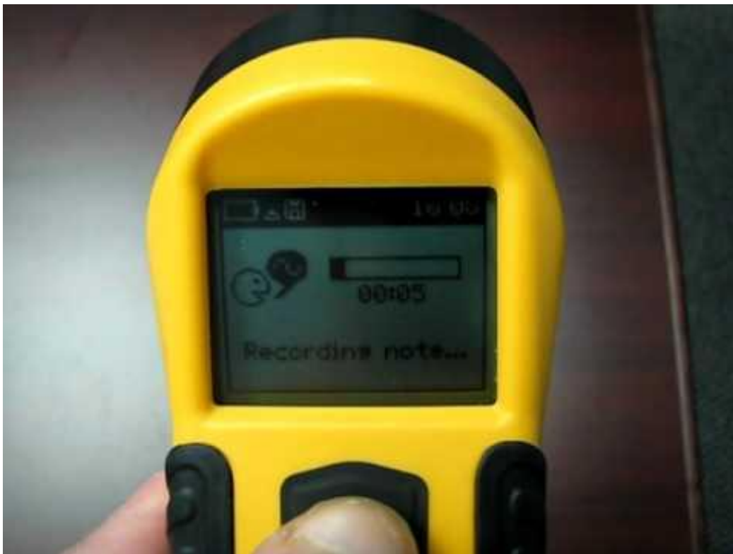
Figure 2.6. Terraplus K-10 Magnetic Susceptibility Meter was used to measure magnetic susceptibilities of rock samples.
