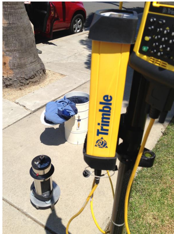
Figure 2.2. Tools were used during our fieldwork. Trimble Pro XRT differential GPS receiver and Worden gravimeter.
